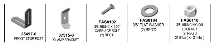
Insert the FRONT STOP POST into the front CROSS SUPPORT and attach with 3/8-16UNCx1.00" CARRIAGE BOLT, 3/8" FLAT WASHER, 3/8-16UNC NYLON LOCK NUT. (Do Not Tighten Yet!).
