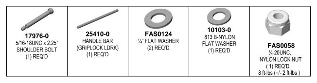
Insert the 2-1/4" SHOULDER BOLT through a  $\frac{1}{4}$ " FLAT WASHER and then through the AXLE. NOTE: the head of the shoulder bolt should face up once the handle bar is attached.
